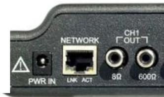
*Pictured: the AUDIO OUT connectors on a professional music on hold player. These are RCA type connectors, and are used almost universally by manufacturers of Music On Hold equipment.*
